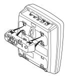
To connect the phone to a two-line phone jack, plug one end of the supplied long two-line modular cord into the TEL LINE 1/2 jack on the back of the phone. Route the cord through the strain-relief slot on the bracket.
